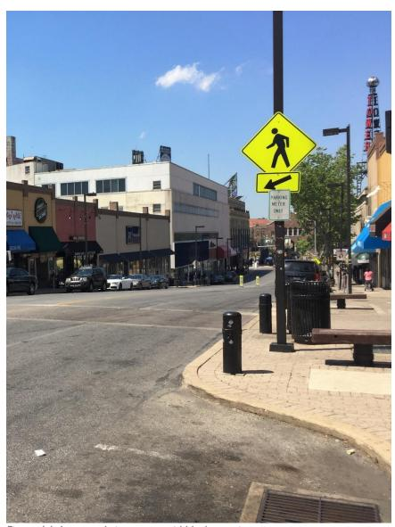
Figure 14: Increased signage at mid-block crossing.
