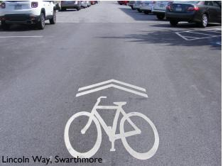
The most common bicycle lane is a striped section of roadway located to the right of moving traffic (left). When the roadway conditions provide enough space, bicycle lanes should be buffered from moving vehicular traffic (top). "Sharrows," which are markers painted on the roadway to delineate where people should cycle, can be used on narrow roadways or streets that have a low volume of traffic (above).
